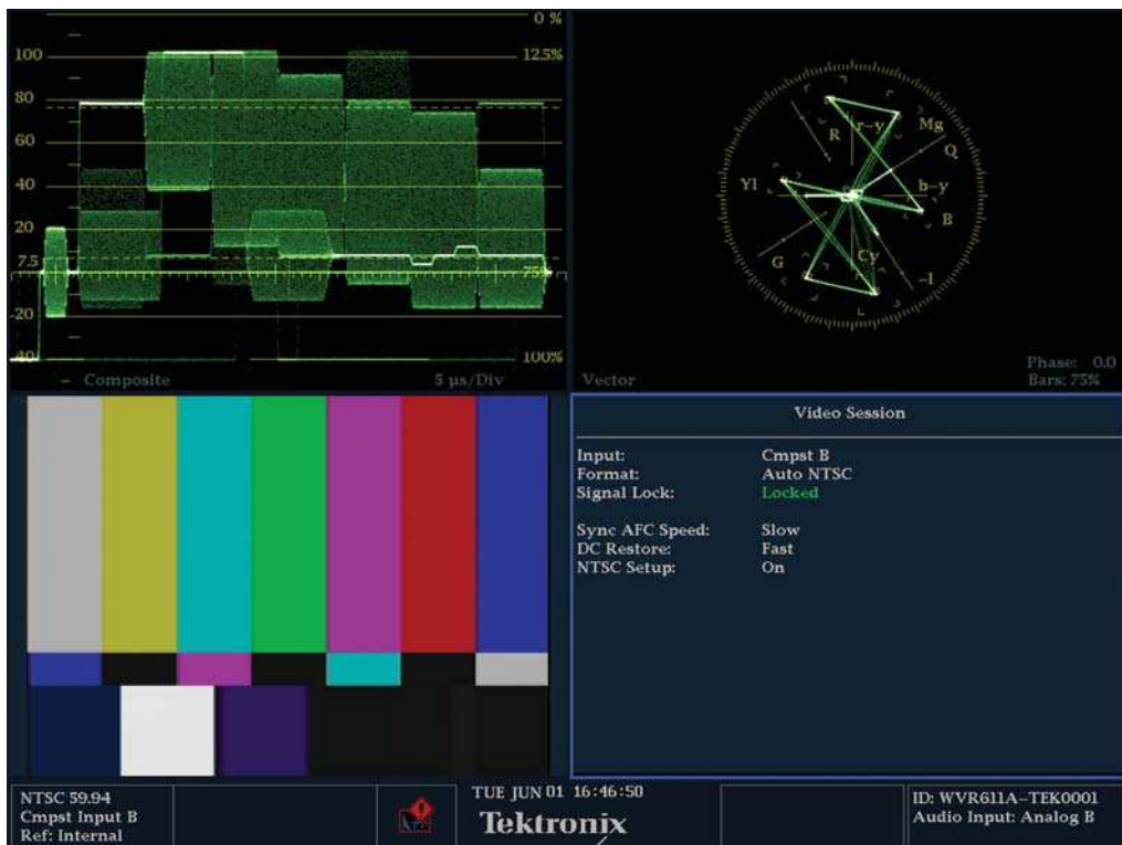
Figure 2.13: Analog component/composite waveform monitor/vectorscope (Photo courtesy of Leader Co.).
