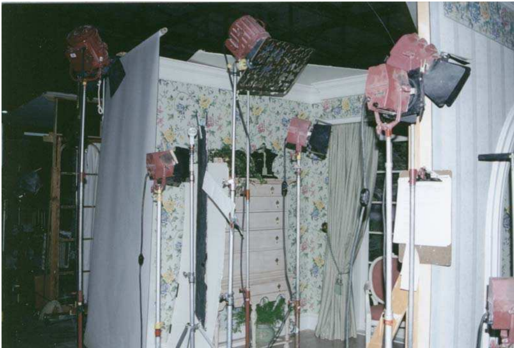
Figure 1.17: Scrim and flags in front of a light source.
