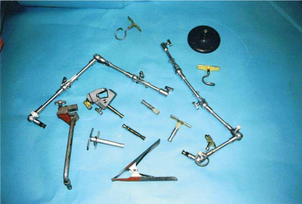
Figure 13.11: Drop ceiling scissor clamp and cable holder.
