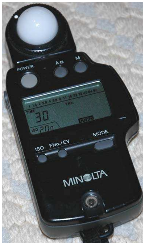
Figure 2.2: Digital incident meter model auto meter VF
