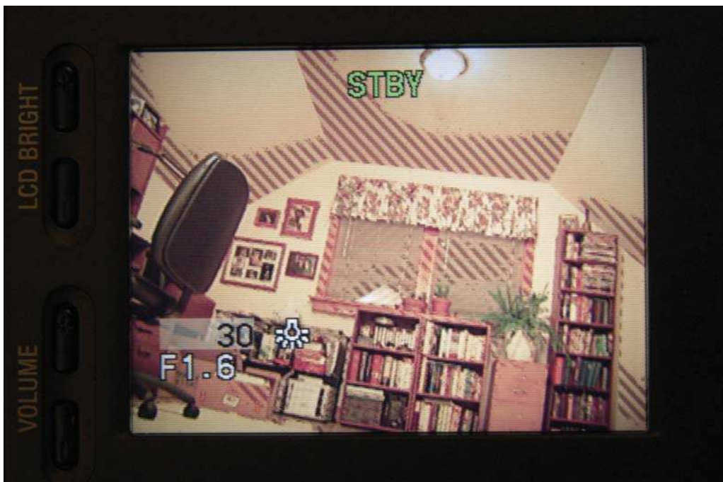
Figure 2.11: Zebra stripes on a DVCAM monitor.
