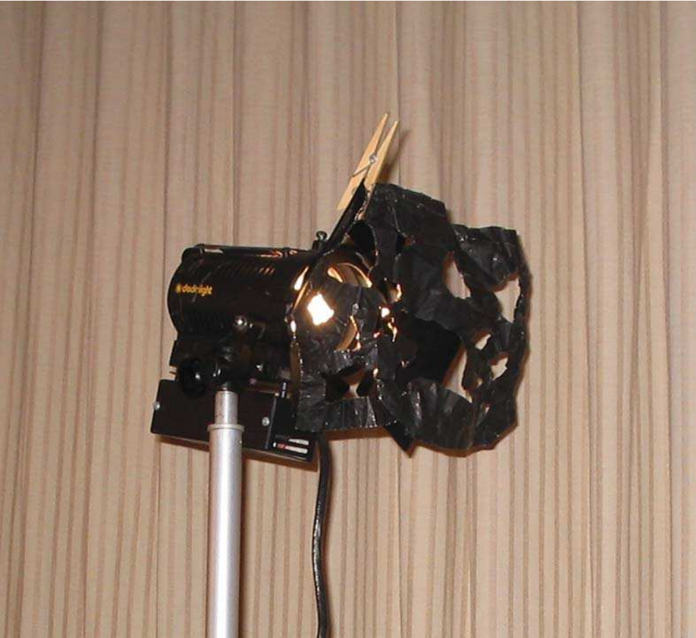
Figure 12.35: Our Dedolight with Blackwrap cookie used as a backlight.
