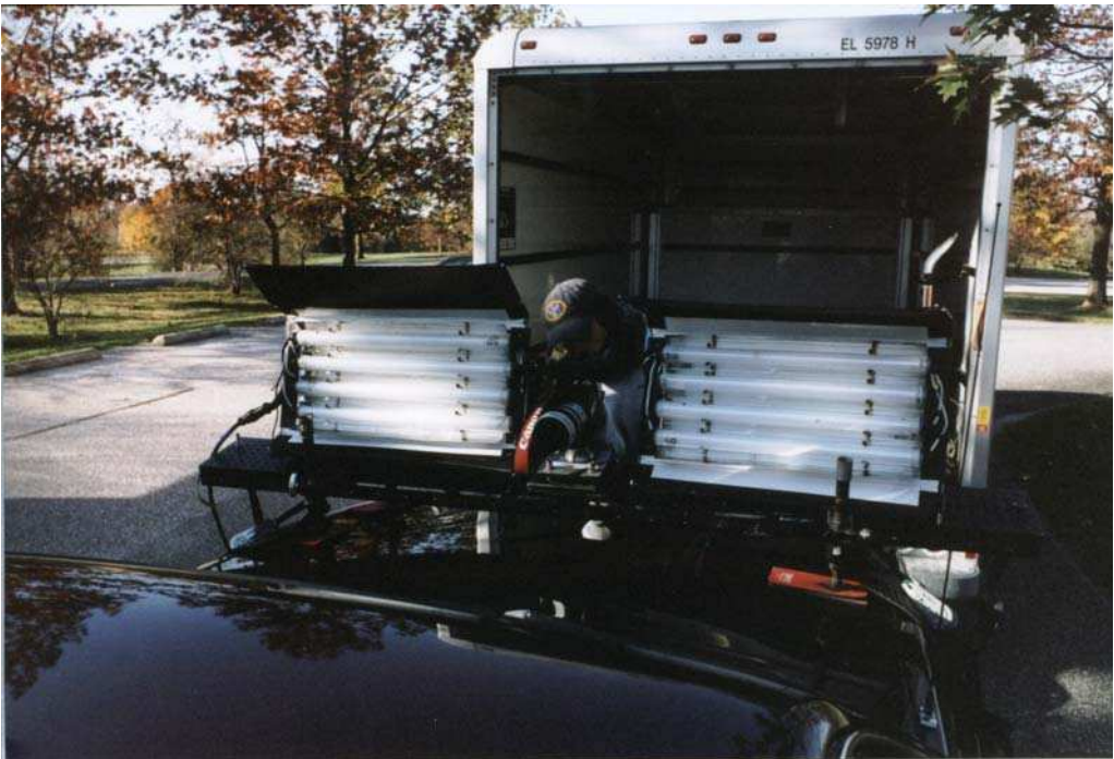
Figure 4.10: Kino-Flo fluorescent lights mounted on a car's hood.
