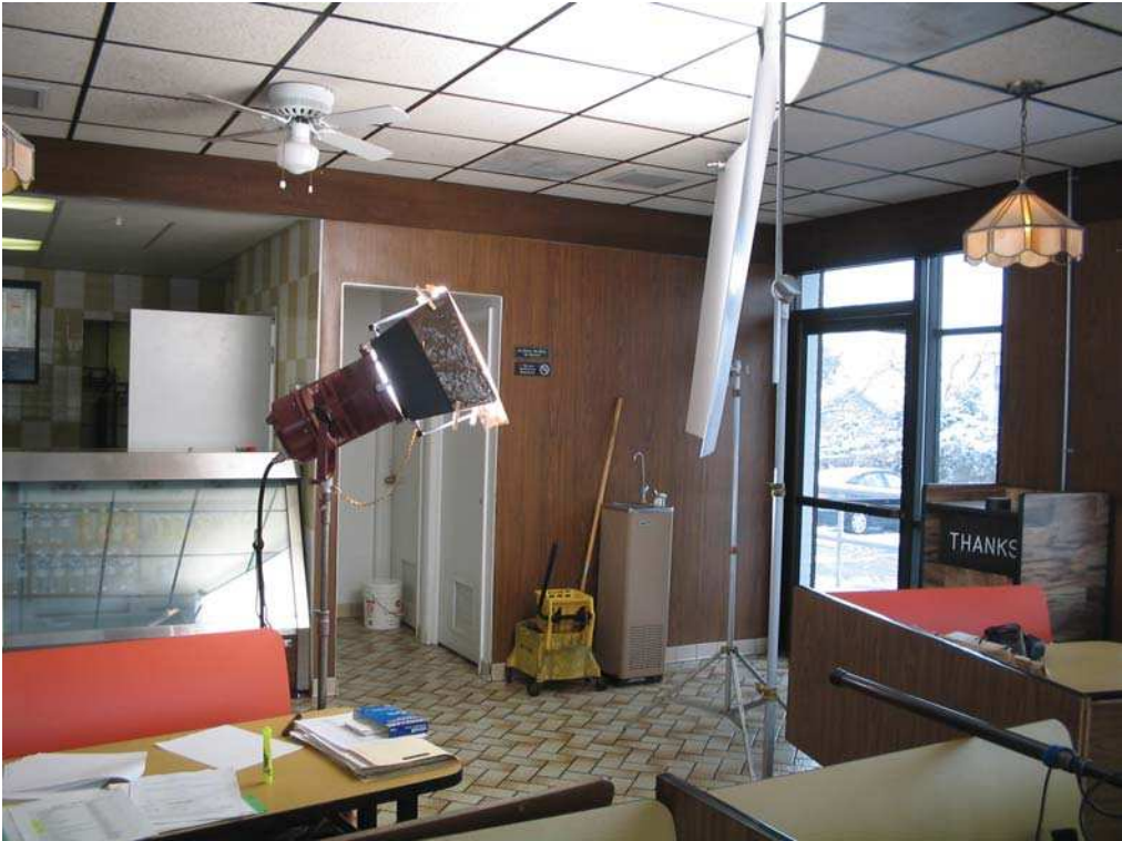
Figure 12.17: An HMI used as a bounce light.
